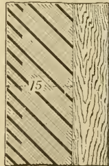
13 in Turret Armor Harveved Nickel Steel Solid.
